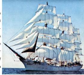
force which drags the ship sideways against the wind. By the use of this and by careful angling of the rudder the ship can make progress towards the wind.
