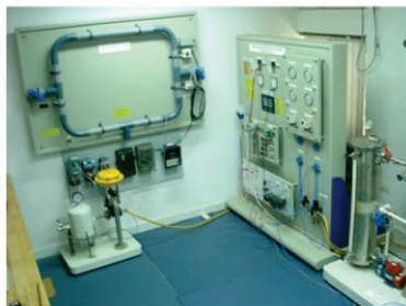
LEFT Automation trainer: An equipment used for Advanced Instrumentation & Process Control course. This program is specially designed to train the ship staff in proper understanding of marine automation systems and instrumentation.
